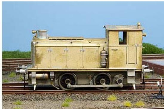
The locomotive viewed from both sides. The air tanks in the kit are too small and they were replaced by bigger ones from brass. Brakes were added and enhanced with extra details. The radiator cap is also an extra detail made by Hans. With some extra work you can turn the kit into a much better model.
