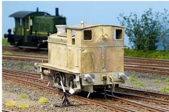
A fellow O gauge modeller, Hans Nijntjes, was able to machine several new parts from brass for me. He made new lanterns, an additional chimney, air tanks and much more. I soldered the chassis and the bigger parts, but I glued the smaller ones. Before you know it adding an extra part means losing a couple of other ones.
