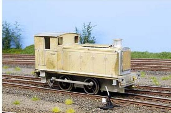
I sand-blasted the model when I was done with the bigger parts. The chassis clearly shows the hole for the hornblocks. As the project progresses it becomes more and more a matter of improvisation. There are quite a few small differences between the locomotives used in The Netherlands and those used in the UK. It is vital to get hold of as much photos of the prototype as you can for reference.
